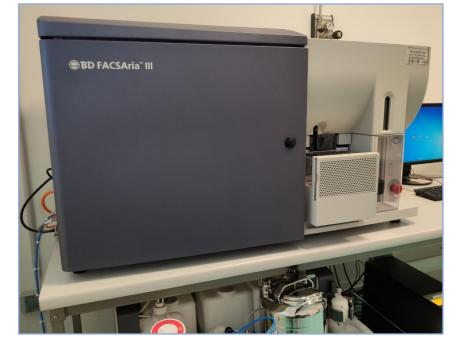
The FACSAria III sorter (BD) performs cell sorting based on a patented technology for a wide range of research applications. Its fluidics and optical systems include laser excitation optics with 5 lasers (355, 405, 488, 561 and 633 nm), a flow cell with gel-coupled cuvette and the octagon and trigon detection systems. It measures up to 18 colors simultaneously, mounts up to 20 detectors and has a maximum acquisition rate of 70000 events/sec.
