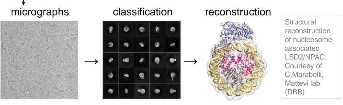
In Cryo-Electron Microscopy (Cryo-EM), through Single Particle Analysis (SPA) hundreds of thousands of images of the isolated particle are collected, classified and used to computationally reconstruct the object in 3D. This technique represents a major breakthrough in the field of structural biology.
